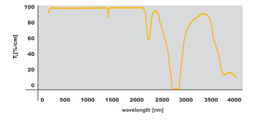
HPFS® Standard Grade is certified to meet T external ≥ 80%/cm@185nm (T internal ≥ 88%/cm@185nm), when measured through a polished, uncoated sample. A typical internal transmittance curve for HPFS® Standard Grade fused silica is shown here.
